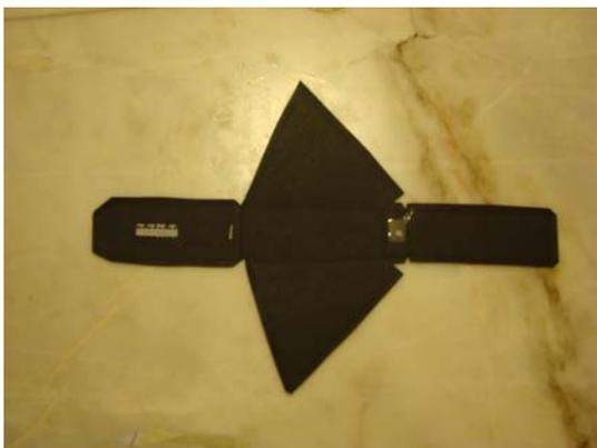
Figure 12. The paperboard after gluing the scale and the diffraction grating
