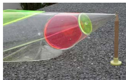
Figure 6. Hyperbolas produced by the Sun and demonstrated together with a model gnomon as conics
